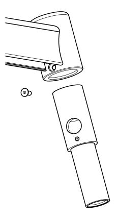
**STEP 2.**Slide adapter into thru post hub from the bottom of the hub. Align mounting hole.
