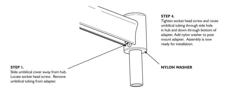
**STEP 2.**Remove socket head screw.
