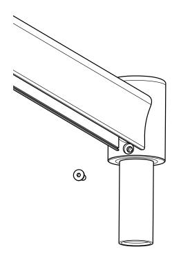
**STEP 3.**Screw in socket head screw.
