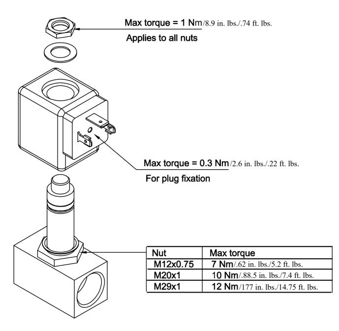
WARNING! Adhere strictly to prescribed torque values. Excessive use of force can cause severe damage to value parts.
