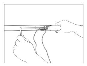
Remove the 4 Flat head screws on the bottom side of the flex arm.
