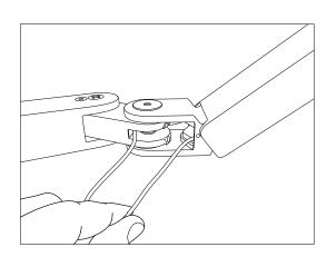
Relieve tension on backside of the flex arm with the Pelton & Crane Spring Tool, DCI PN 8697. Do not back the screw all the way out, only until the tension is relieved from the spring.
