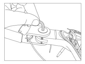
Pull out the wiring from the back side of the flex arm. Do not remove the wires from the transformer side.
