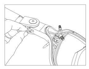
Back out the 2 set screws on the side of the knuckle that retain both the top and bottom snubbing pins.
