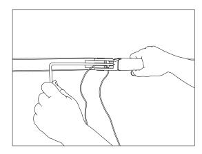
Pull the arm to the horizontal position. Once the tension screw lines up with the drilled hole insert a 9/64 hex wrench to adjust drag.
