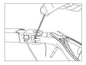
Unscrew the bottom and top snubbing pins. Be sure to hold light head during removal.
