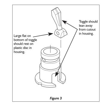
The remaining parts in the kit are for use in rebuilding the foot control valve, located under the chrome foot control disc.
