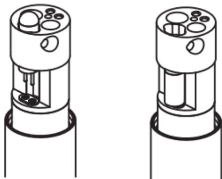
If the LED does not illuminate when activated remove bulb, rotate 180°, and re-install.
