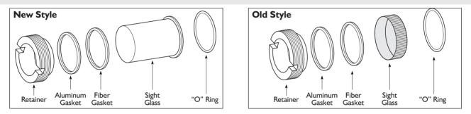
To install the new sight glass assembly, insert the "O" ring gasket, making sure that it is evenly seated in the sight glass spud. The "O" ring must be oiled before insertion. Screw in the sight glass assembly to contact the "O" ring and torque to specification. Torque 90 to 110 inch pounds maximum.
