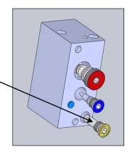
Turn on all pressure supplying devices. Remove appropriate handpiece from holder, activate foot control and verify handpiece function as well as water coolant to handpiece. Hang up handpiece in holder, checking that holdback function is operating, and activate handpiece; there should be no flow of air or water to handpiece. Verify no leakage of air or water of replaced components. System is now ready for use.
